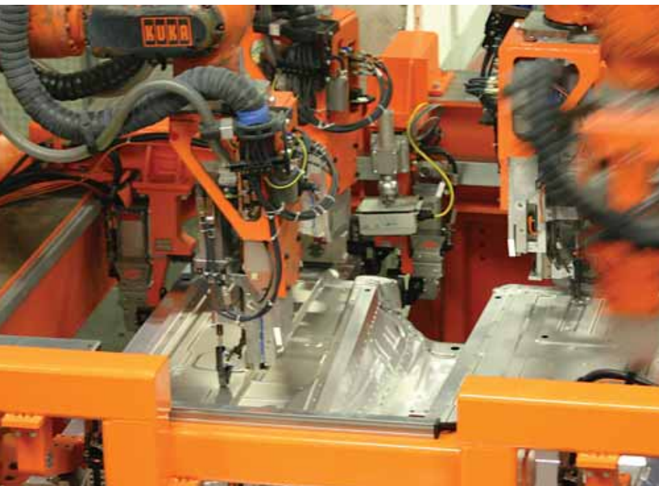
Audi AG has used the RSF20S screwdriving system to assemble chassis and body panels for many of its models since 1996. Photo courtesy Weber Screwdriving Systems
